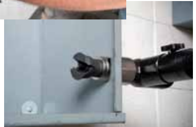
Fix the die and start punching.
