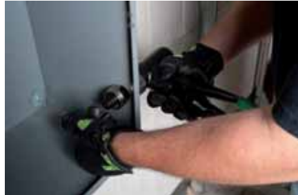
Fix the die and start punching.
